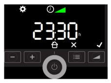
The keys of the device may have different functions. If there is a symbol above the key in the display (e.g. **3** above the softSTART key), the key adopts the function of the symbol in question. If there is no symbol above the key (e.g. in the case of the key), the key retains its original function.
