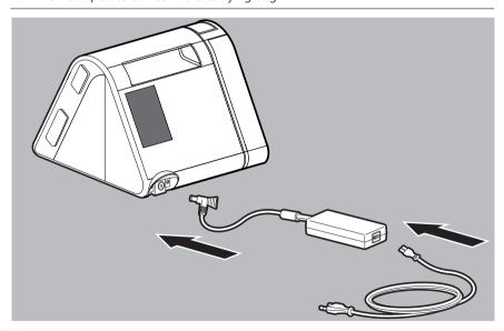
1. Connect the power supply unit to the device.
