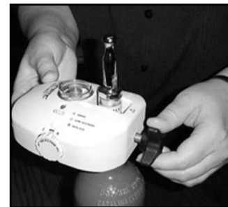
FIGURE F Attaching the OXYMATIC® conserver to the cylinder
